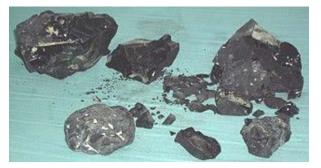
capture oil sand tailings containing a mixture of salts, suspended solids and dissolvable chemical compounds and toxic hydrocarbons produced as a byproduct of bitumen extraction from the oil sands. Managing these tailings is one of the most difficult environmental challenges facing the
