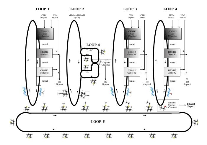
The above schematic of a hypothetical mechanosynthetic production line for ethanol molecules (black = C, white = H, yellow = Ge, red = O, blue = metal or Ge surface) has inputs of methane (CH<sub>4</sub>) and water (H<sub>2</sub>O) and outputs of ethanol (C<sub>2</sub>H<sub>5</sub>OH) and hydrogen gas (H<sub>2</sub>). The production line consists of six interacting continuous or stepwise-moving conveyor loops as described below.
