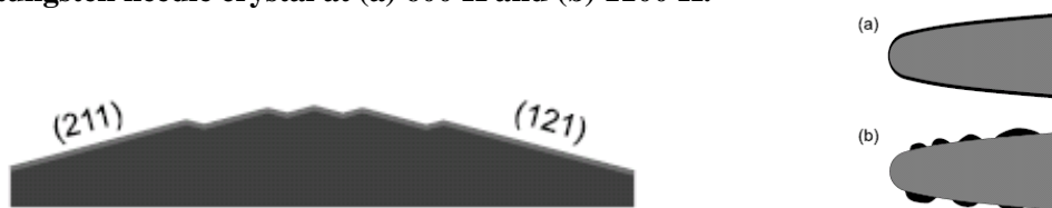
Figure 5-12. Left: Schematic model of the tungsten crystal faceted by the presence of Pd, viewed in cross-section. Right: Schematic drawing illustrating Pd distribution on a tungsten needle crystal at (a) 600 K and (b) 1100 K. 515
